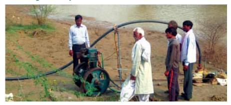
Five Lift Irrigation Systems (LIS) was installed for four check dams built by PHDRDF with support from various donors. This intervention provided the farmers easy and timely access to the water reservoir enabling them to irrigate their farm lands and thereby increasing their agricultural yield.
